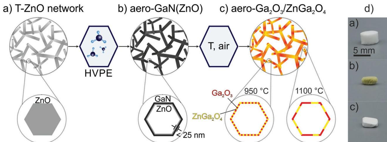
**Figure 1.** Sample photographs and schematic of the two-step synthesis process of gallium oxide-based aero-networks. a) Macroporous networks of interconnected ZnO tetrapods are used as sacrificial templates for the HVPE growth of b) aero-GaN(ZnO) networks which are transformed into hybrid nanocomposite structures of c)  $\beta$ -Ga<sub>2</sub>O<sub>3</sub>/ZnGa<sub>2</sub>O<sub>4</sub> with annealing at 950 and 1100 °C. d) Photographs of the physical network structures.
