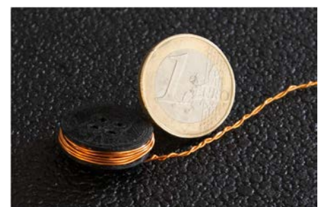
Figure B9-3: Electric coil designed as a small button, which can be easily sewn to garment.
