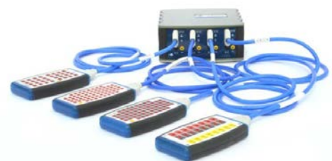
Fig. B10-5: ECG system “g.Hlamp-RESEARCH” from g.tech with 144 electrodes [Picture source: g.tec].
