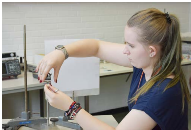
Fig. SOP-3: A simple and low-cost experiment for the qualitative and quantitative investigation of magnetostrictive characteristics, employing magnetostrictive laser deflection and optical amplification (left) and a magnetoelectric sensor built by a student as part of the out-of-school project day (right).
