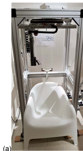
Figure Z2-13: (a) Pneumatically driven head scanner with telescopic arm for the measurement on phantoms and patients. The scanner is made of non-magnetic materials for operation in a magnetically shielded chamber. (b) Rack with laboratory equipment for generating test signals for the phantoms, multichannel data acquisition hardware (2 professional sound cards RME Fireface UFX+), and powerful workstation for digital signal processing.
