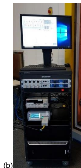
Figure Z2-13: (a) Pneumatically driven head scanner with telescopic arm for the measurement on phantoms and patients. The scanner is made of non-magnetic materials for operation in a magnetically shielded chamber. (b) Rack with laboratory equipment for generating test signals for the phantoms, multichannel data acquisition hardware (2 professional sound cards RME Fireface UFX+), and powerful workstation for digital signal processing.
