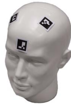
Figure Z2-17: Head phantom with “ArUco” digital markers for position estimation
